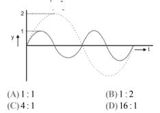
11. The equation of displacement of two waves are given as  $y_1 = 10 \sin (3\pi t + \pi/3)$  and  $y_2 = 5(\sin 3\pi t + \sqrt{3}\cos 3\pi t)$ , then what is the ratio of their amplitude:-
